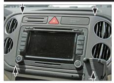
Unclip and remove OEM panel 1. (see arrows)
