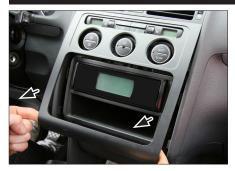
1. Unclip and remove OEM panel (see arrows)
